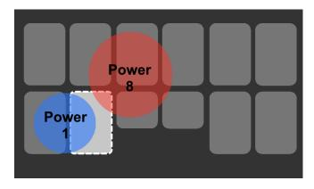
Due to safety reasons, the pan with the lowest power level has priority (blue pan – power [ 1 ]). This means that the induction coil with the conflict (marked in white) will only transmit the power which is necessary to get the requested power level of this pan.
